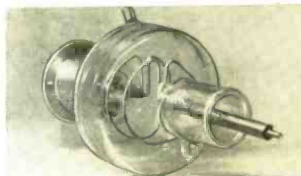
Fig. 3—The insulated r.f. coupling system.
