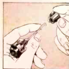
U-clip furnished to slide over end of shaft—holds set-screw knobs.
